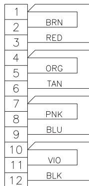
WIRING DIAGRAM ADDRESS PLUG WITH ALL WIRES CONNECTED
